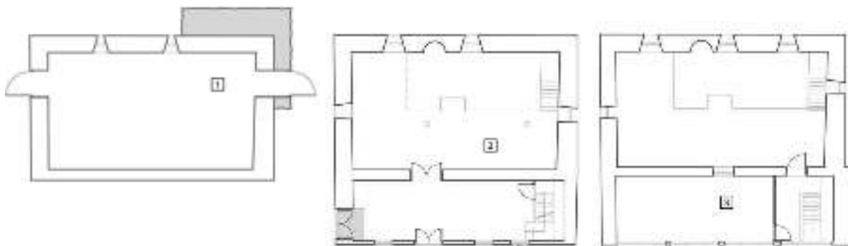
Figure 2: Plan of basement (1), ground floor (2) and the first floor (3) of Kučanska Mosque
