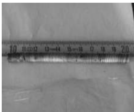
Figure 6: Wood core extracted from a beam.
